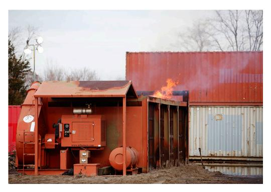
Note and Credits: The US Army Corps of Engineers performing an Air Curtain Burning of over 77,000 cubic yards of vegetative debris, mostly tree branches downed by Hurricane Sandy at Floyd Bennett Field in Brooklyn, N.Y., Nov. 28, 2012. Source: Chris Kleponis, <a href="https://www.dvidshub.net/image/790740">https://www.dvidshub.net/image/790740</a>
